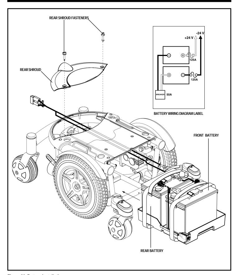
Figure 26. Battery Installation
